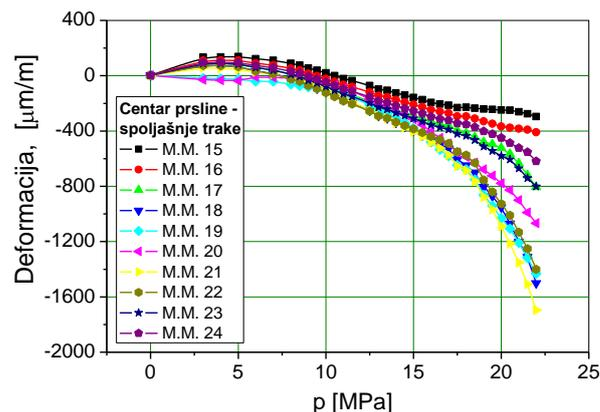
Fig. 5: Dependence of the strain from pressure, inner straps - middle of crack
