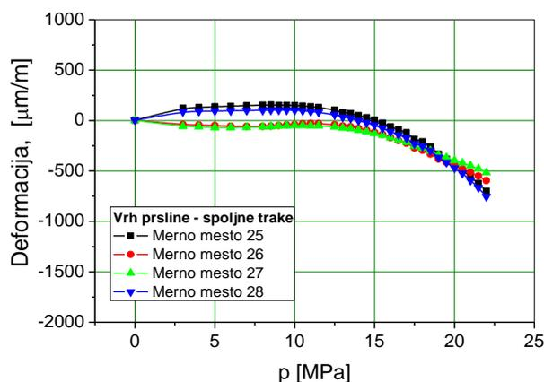
Fig. 7: Dependence of the strain from pressure, outer straps - crack tip
