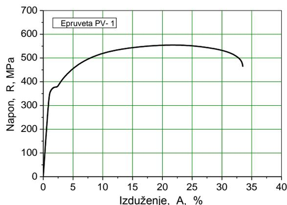
Fig. 1: Diagram of stress – percentage elongation, test tube PV-1, tube from exploitation, 20 °C
