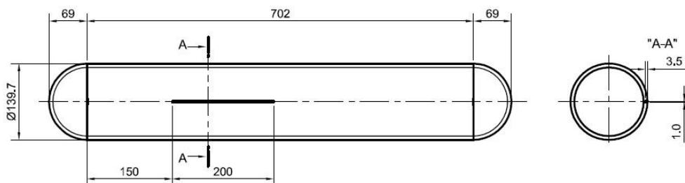
Fig. 2: The vessel with an axial surface crack on the outside
