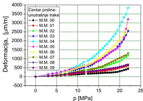
Fig. 4: Dependence of the strain from pressure, inner straps - middle of crack
