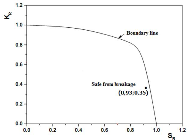
Fig. 8: Fracture analysis diagram (FAD) for tube
