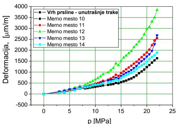
Fig. 6: Dependence of the strain from pressure, inner straps - crack tip
