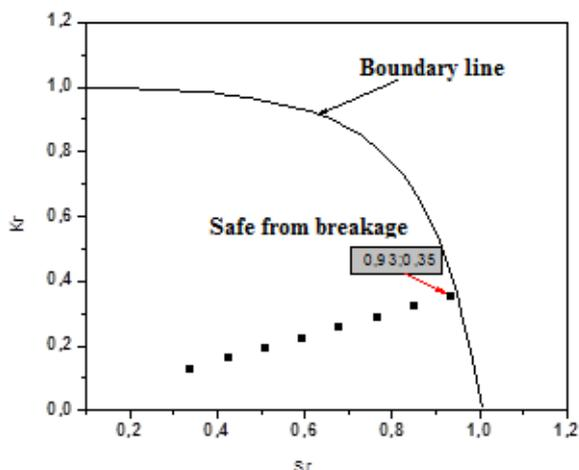
Fig. 9: Fracture analysis diagram (FAD) for tube With an axial surface crack on the outer surface at various pressures
